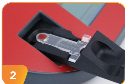
2 Put microcuvette into analyzer.
