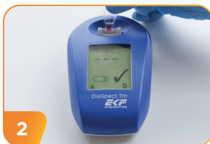
2 Insert the filled cuvette and press down gently. Remove the cuvette immediately after the first beep tone.
